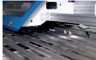
Indexed conveyor for magazining the material bar profiles in a defined position
